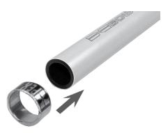
• Insert a PEX fitting into tube up to the fitting shoulder and position the crimp ring 1/8" to 1/4" from end of pipe. To prevent ring from moving, squeeze the ring slightly with your fingers or a pair of pliers.
