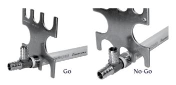
Joints that do not pass the gauge check must be cut out and replaced. DO NOT RECRIMP (Double Crimp) THE SAME FITTING.
