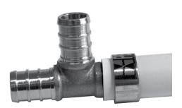
Ocenter the crimping tool exactly over the ring, and keeping both the ring and the tool square with the tube, close the tool completely.
