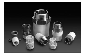
Transition fittings are available for connecting to other materials, valves and appurtenances and must be used for all hot water line connections. For cold water connections, male CPVC threaded adapters may be used. They are not recommended for hot water use as wide temperature fluctuations can result in a drip leak.
