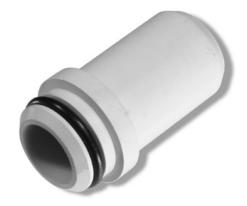
Standard compression fittings which utilize brass ferrules can be used on CPVC, although we recommend the use of an O-ring transition (above). If a brass ferrule is used, Teflon® tape must be applied over the ferrule to compensate for the dissimilar thermal expansion rates of the brass and CPVC that could possibly result in a drip leak. Care should be exercised not to over-torque the compression connection.
